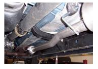
INSTALL HEAD PIPE #A ON TO YOUR EXISTING STOCK 2-BOLT FLANGE AND SECURE WITH BOLT KIT #F. INSERT WELDED HANGER INTO RUBBER GROMMET. DO NOT TIGHTEN
