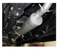
INSTALL MUFFLER #B ONTO HEAD PIPE 1-1/2" TO 2" WITH THE LOUVERS FACING TOWARDS THE CONVERTER. THE MUFFLER OUTLET SHOULD BE POSISTIONEDTHE MUFFLER OUTLET SHOULD BE POSITIONED AT 12:00. USE A JACK STAND TO SUPPORT THE MUFFLER. USE CLAMP #E TO SECURE THE MUFFLER TO THE HEAD PIPE. DO NOT TIGHTEN. MUFFLER INLET IS LOOKING INTO THE LOUVERS.
